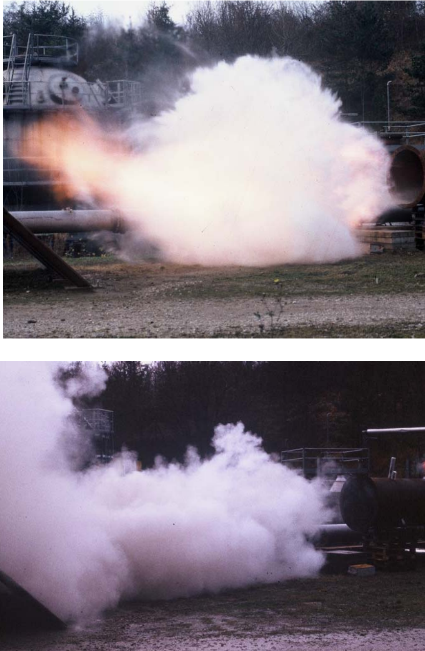
Figure 12. Dust explosion (St 1) in a pipeline DN 1000 (above without, below with extinguishing barrier
