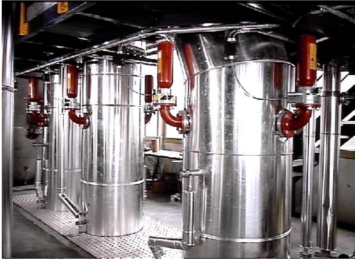
Figure 11. Extinguishing barrier in connecting pipes
